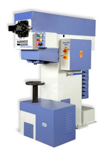
Machine designed with fully automatic loading, measuring and unloading cycle. A compact hydraulic power pack and control circuit with built in optical device with 14X magnification provided in front to project diameter of ball impression on glass screen with micrometer measuring system with 0.01 mm least count. **Features:**
